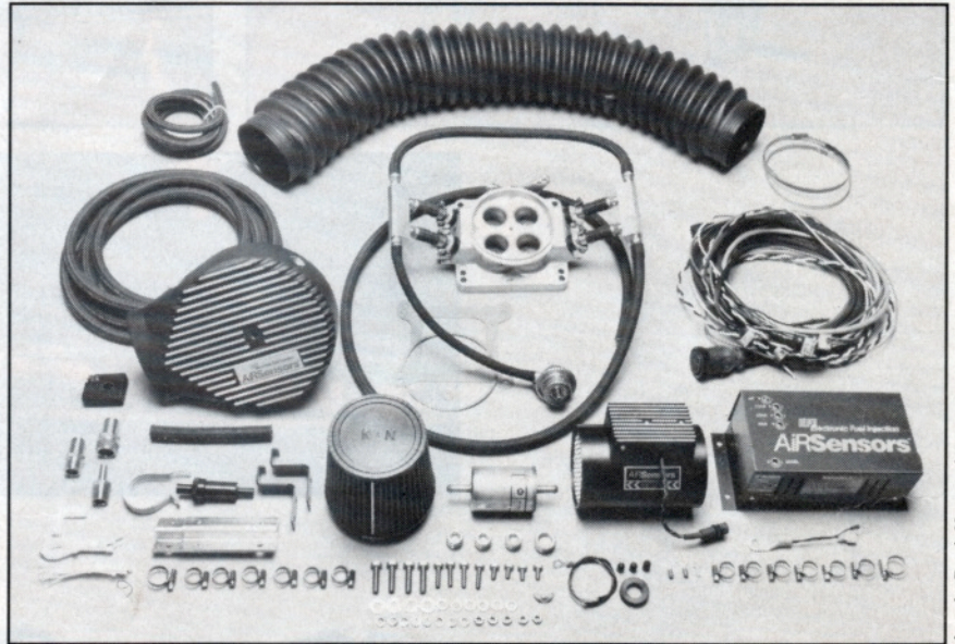
The AirSensors system, suitable for a variety of engines, was installed on a Chevy 454 (right) for evaluation. System relies on air-mass sensor and electronic control to correctly meter fuel.
